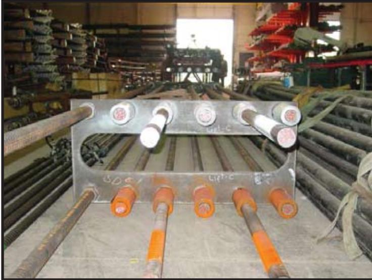
Color coding the thread bars and couplers on the prefabricated cages makes installation easier for the workers at the job site.
